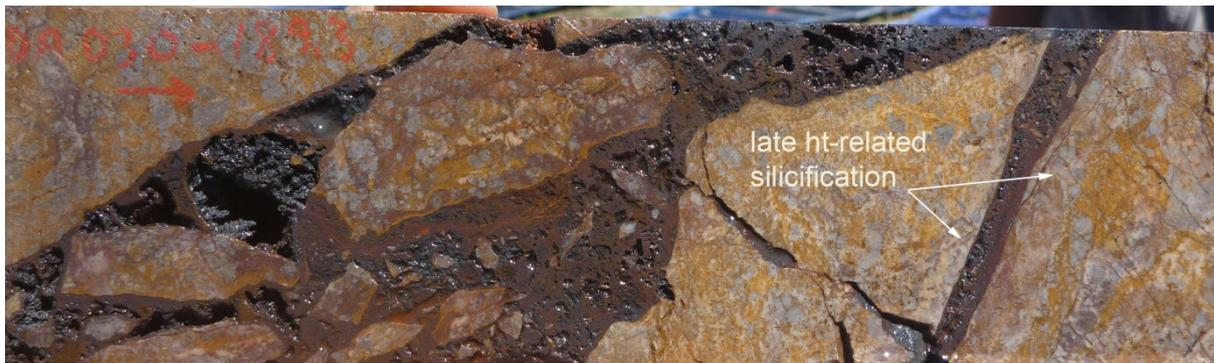
Figure 13. Typical hematite-matrix mosaic breccia veins, carrying good gold grades (Erato). These features show evidence for the commencement of high energy hydraulically-driven clast transport. They overprint the already hydrothermally brecciated and silica-cemented Upper Volcanics, and a generation of silica alteration is associated with the hematite. Late limonite overprints locally.
